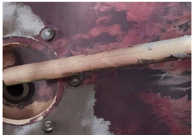
Above: The gas tank windows and cracks in pick up tube. Repairing the cracks fixed the problem.
