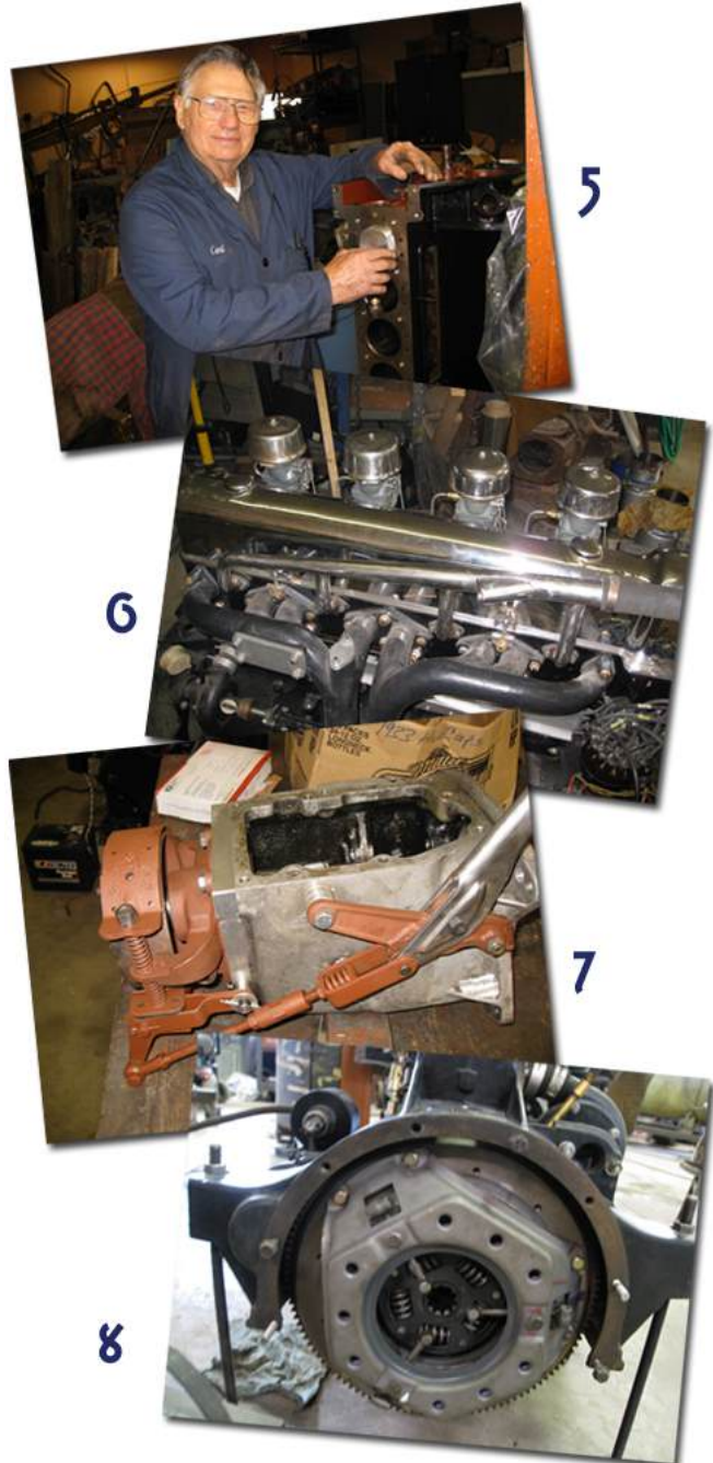
Top to Bottom: 5) Carl installing the new pistons. 6) Flywheel modifications to accept 11 inch high performance Ford clutch and pressure plate. 7) 1984 Ford Truck transmission with overdrive modified to fit Stutz. 8) The finished engine ready to go. The four carb manifold was replaced with a two carb manifold during the dialing-in process.
