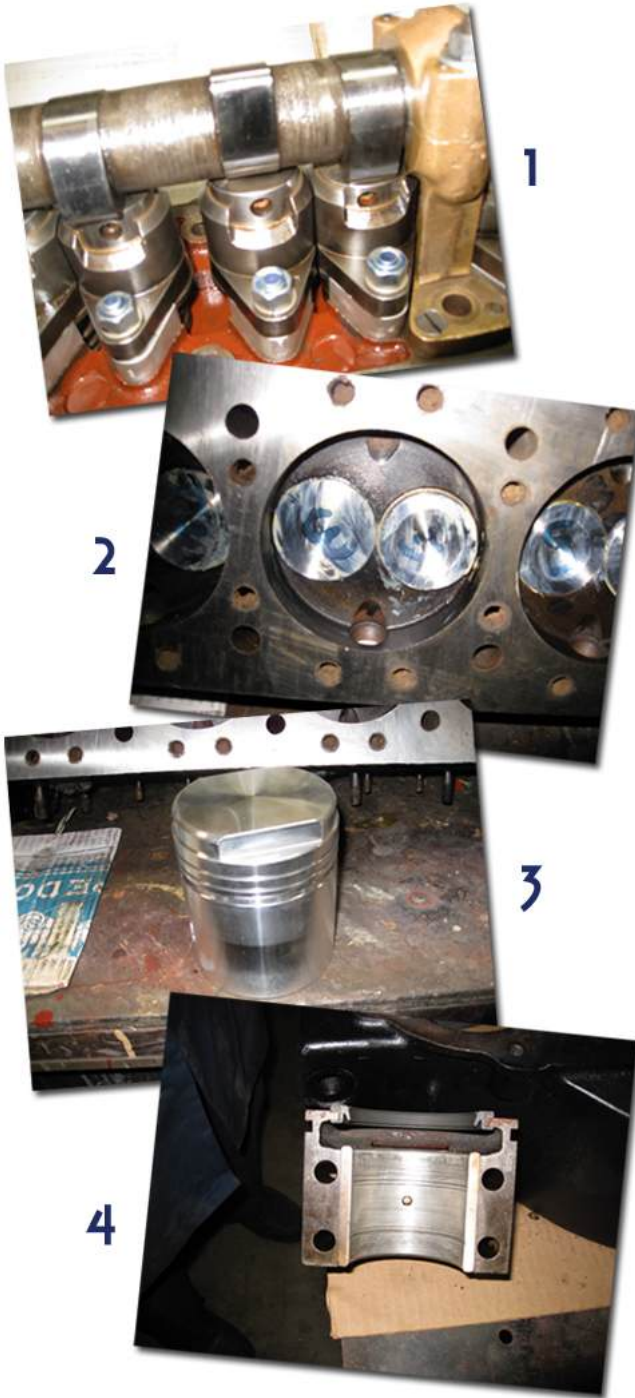
Top to Bottom: 1) Chevy Vega lifter upgrade with the revised cam regrind. 2) Enlarged intake and exhaust valves installed into the ported head. 3) Arias Piston with 10.5:1 compression ratio. 4) Chevy Big Block rear main oil seal installed into the Stutz block.
