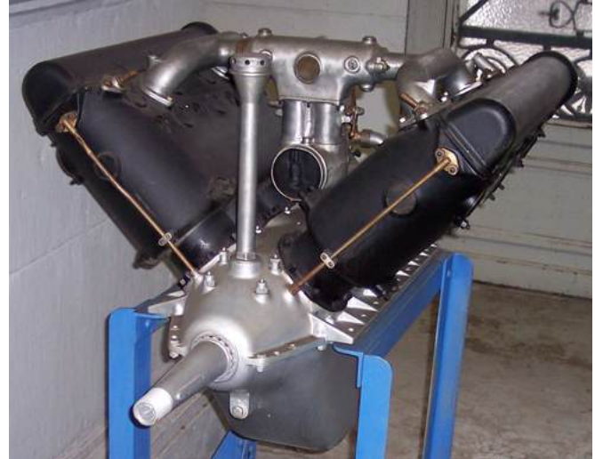
Hispano-Suiza HS.8A SOHC WWI aviation engine with overhead camshafts, preserved in a Brussels museum. Photo credit: Stahlkocher, CC-BY-SA-3.0
